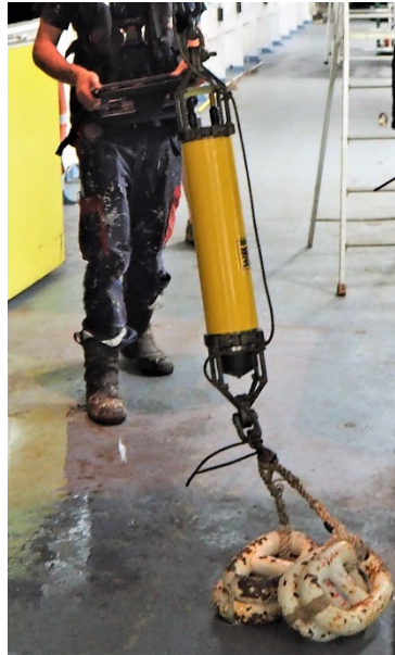
Figure 14: UTM's Emergency Recovery Beacon (ERB) prepared for deployment with anchor weight.
