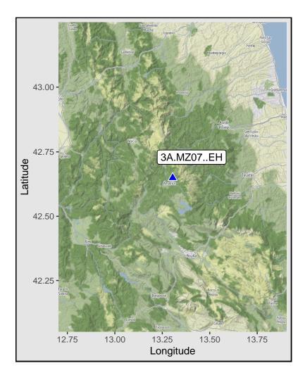
Station: MZ07, Net: 3A, Loc: (S-Phases: 2552, Noise:746) Start: 2016-09-20, Mag min: 0.1 - Mag max: 4.3
