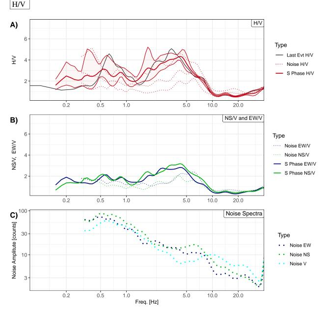
Station: CSD, Net: 4A, Loc: 01 (S-Phases: 6, Noise:6) Start: 2013-10-08, Mag min: 2.7 - Mag max: 3.3 Last event: CS (Scalea), 2013-12-10 20:39:39, MI:2.7 [INGV]
