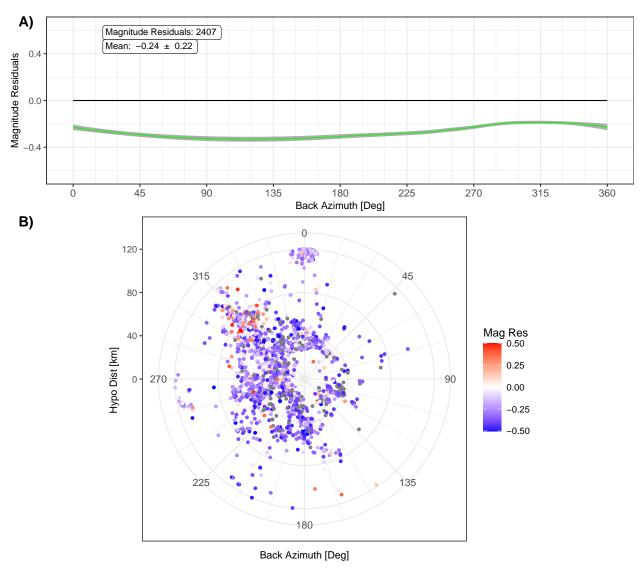
Local Magnitude Residuals (single station magnitude - averaged event mganitude). Magnitudes were calculated using the relation given by Di Bona (2016) without taking into account for station corrections. A) magnitude residuals versus distance (mean). B) magnitude residuals as function of distance and back azimuth.
