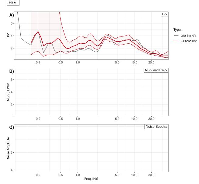
H/V and noise spectra. Spectral ratios are computed considering both S-phase and noise windows, as indicated in the legend. A) H/V for the horizontal (H) component, the average  $\pm$  one standard deviation of the ratios computed for several windows are also shown and the gray line (Figure A) is the H/V relative to the last automatically processed seismic event. B) H/V for the EW and NS components (mean). C) noise spectra (mean).
