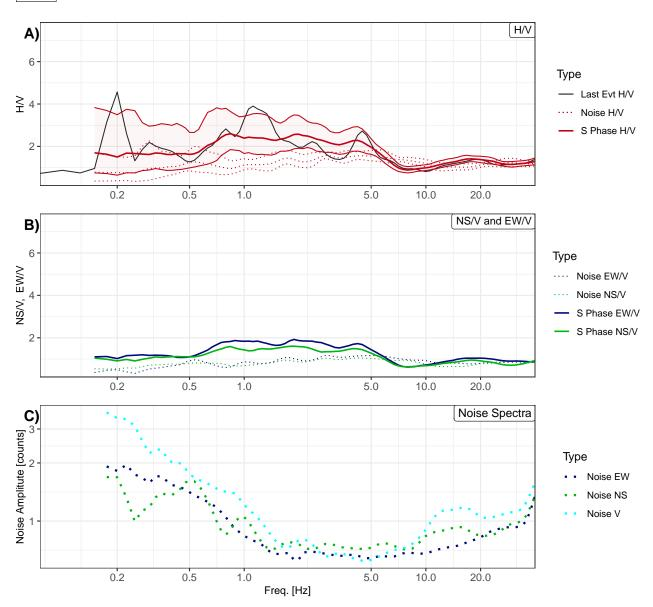
H/V and noise spectra. Spectral ratios are computed considering both S-phase and noise windows, as indicated in the legend. A) H/V for the horizontal (H) component, the average ± one standard deviation of the ratios computed for several windows are also shown and the gray line (Figure A) is the H/V relative to the last automatically processed seismic event. B) H/V for the EW and NS components (mean). C) noise spectra (mean).
