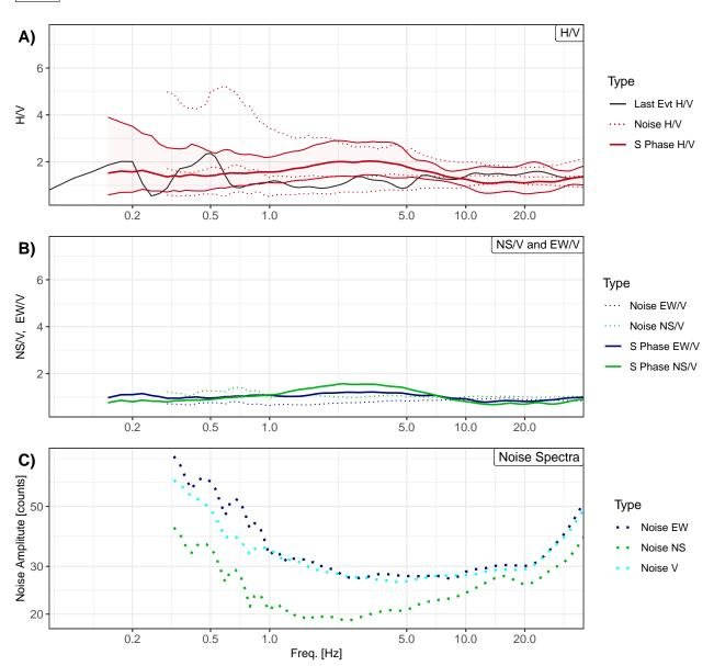
Station: SGMA, Net: IT, Loc: (S-Phases: 167, Noise:145) Start: 2013-12-20, Mag min: 0.9 - Mag max: 6.2 Last event: Lucera (FG), 2024-01-24 01:29:44, MI:1.9 [INGV]
