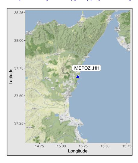
Station: EPOZ, Net: IV, Loc: (S-Phases: 668, Noise:701) Start: 2013-03-21, Mag min: 1.5 - Mag max: 4.8
