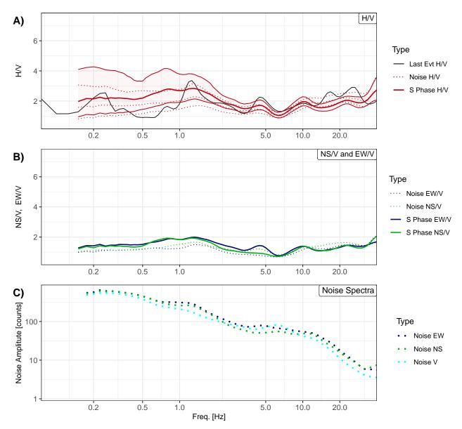
H/V and noise spectra. Spectral ratios are computed considering both S-phase and noise windows, as indicated in the legend. A) H/V for the horizontal (H) component, the average  $\pm$  one standard deviation of the ratios computed for several windows are also shown and the gray line (Figure A) is the H/V relative to the last automatically processed seismic event. B) H/V for the EW and NS components (mean). C) noise spectra (mean).
