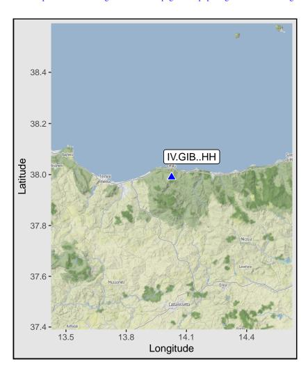
Station: GIB, Net: IV, Loc: (S-Phases: 692, Noise:679) Start: 2012-01-01, Mag min: 1.5 - Mag max: 4.8 Last event: Troina (EN), 2023-01-28 15:26:32, MI:2.2 [INGV]
