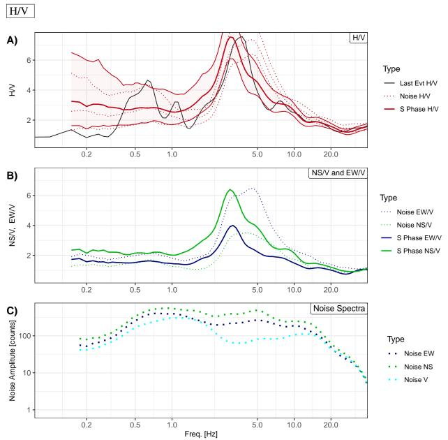
Station: OT13, Net: OT, Loc: (S-Phases: 208, Noise:154) Start: 2019-07-19, Mag min: 0.9 - Mag max: 3.9 Last event: FG (Isole Tremiti), 2023-06-15 04:28:07, MI:1.8 [INGV]
