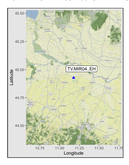
Station: MIR04, Net: TV, Loc: (S-Phases: 1203, Noise:1392) Start: 2012-05-24, Mag min: 0.5 - Mag max: 5.6 Last event: Bondeno (FE), 2012-07-16 17:39:03, Ml:2.9 [INGV]
