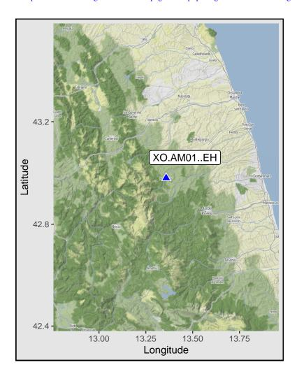
Station: AM01, Net: XO, Loc: (S-Phases: 4023, Noise:1649) Start: 2016-08-29, Mag min: 0.2 - Mag max: 4.6
