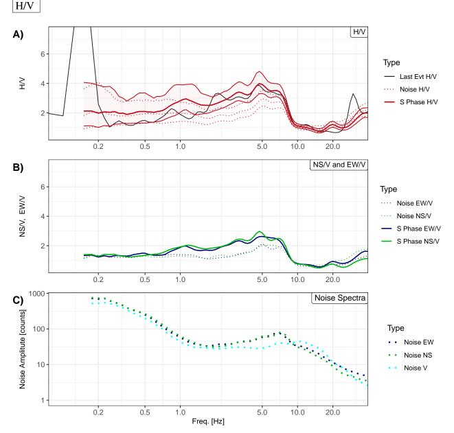
Station: A280A, Net: Z3, Loc: (S-Phases: 117, Noise:151) Start: 2015-09-24, Mag min: 1.1 - Mag max: 4.2 Last event: Sampeyre (CN), 2018-12-24 00:01:52, MI:2.4 [INGV]
