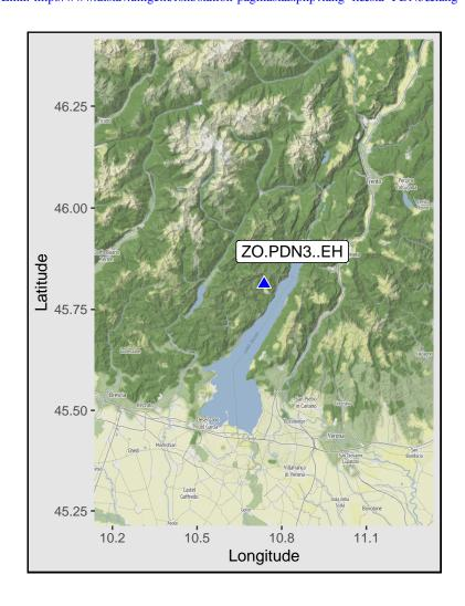
Station: PDN3, Net: ZO, Loc: (S-Phases: 15, Noise:14) Start: 2022-01-17, Mag min: 1.5 - Mag max: 4.3
